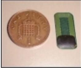
Size of the LTO-CM inside the Cleaning Cartridge.
